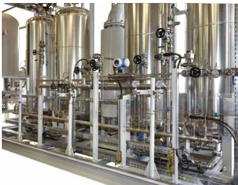
Fig. 3 - Close-up of PSA oxygen generation plant
